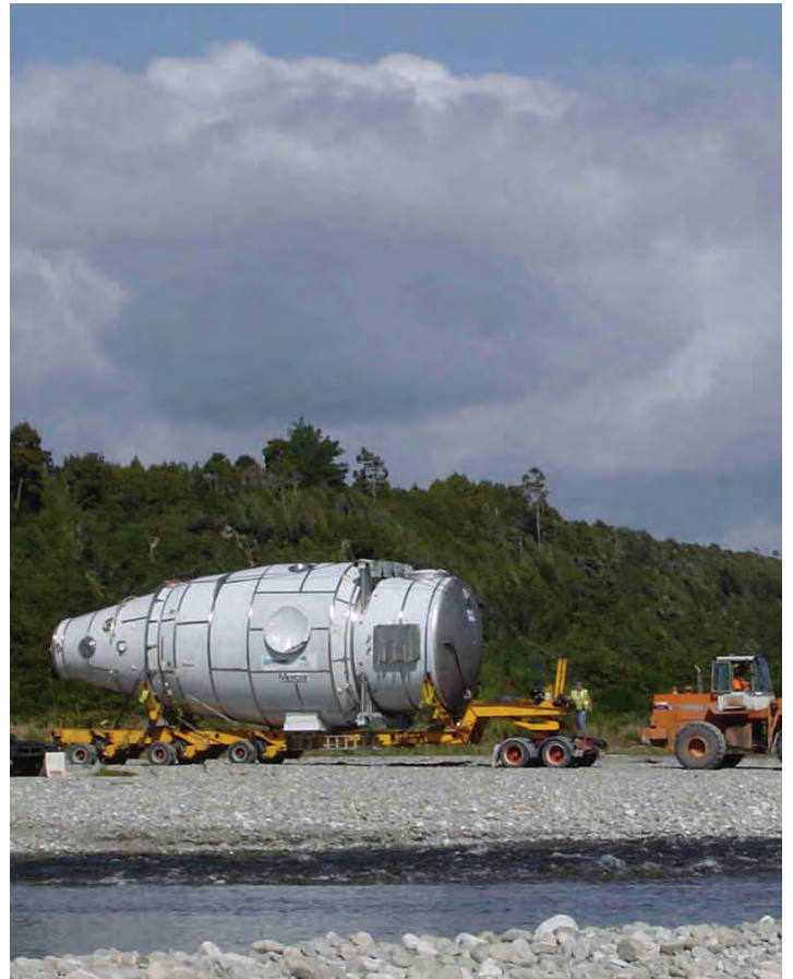
An exceptional transport of a CIP filter
